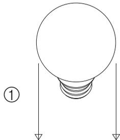
① Once all parts have been removed from box along with any protective packing, install an UL listed E-26 LED lightbulb (not included) into the lampholder within the luminaire. Use only lightbulbs that do not exceed the maximum wattage rating. (25W)
